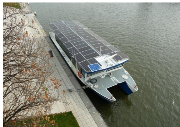
Figure 69 Electric solar ship "Wolfsburg 2". The solar panels are the range extender here. [106]
