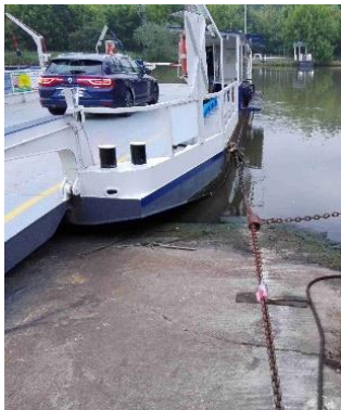
Figure 5 Guide chain of a chain ferry across the Saale river. [9]
