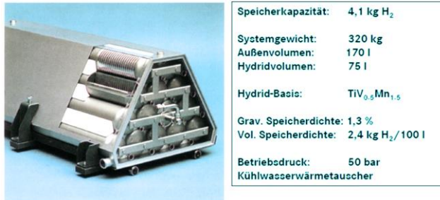
Figure 60 Metal hydride storage for hydrogen. [97]
