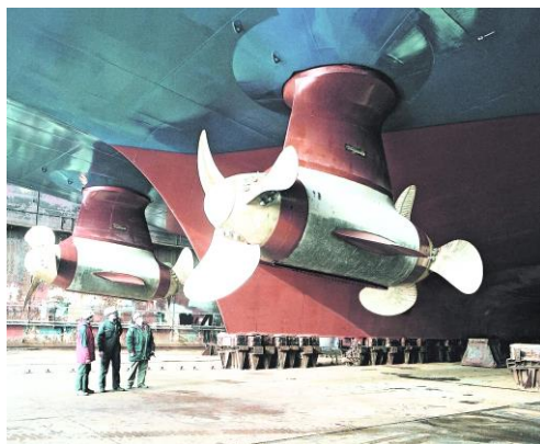
Figure 38 Two pods (Siemens Schottel Propulsor) for ferries. [68]
