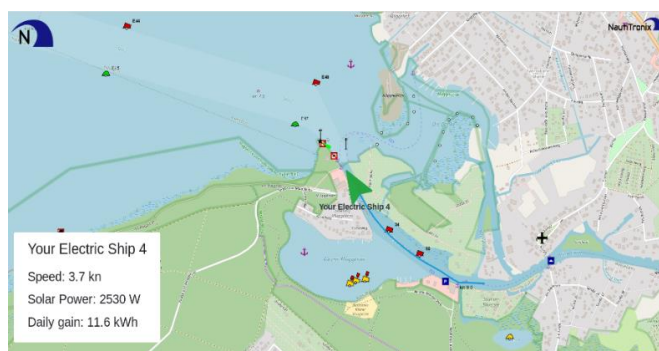
Figure 92 Passenger information with position, speed and power for an electric ship. [121]
