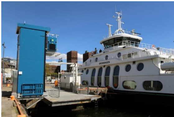
Figure 9 Electric ferry "Dronningen" at the fast charging tower, Oslo harbour. [13]
