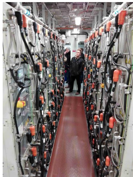
Figure 45 View into the battery compartment of the M/F "Elektra". The lithium-ion battery has a total charge of 2 \times 500 \text{ kWh} . [78]
