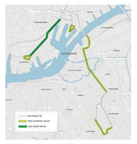
Map of Bus Route 55 showing in which areas the zone management system is set to electric drive and where max speed is limited. Dark green shows low speed zones. Light green shows zreo emission zones.
